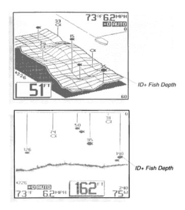
"ID+", the default setting, provides more information about the location of the target by attaching depth "strings" showing the digital depth of the target. When there are numerous targets onscreen, not every target depth is shown, to avoid excessive clutter on-screen.
